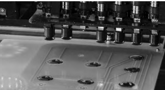
Automated Dome Placement
